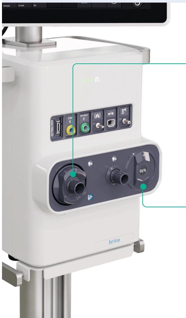
The **Expiratory Port** has been specially developed for a more direct and precise electronic control of the respiratory phases of the breathing cycle. It enables an improved response time and the spontaneous breathing of the patient even during the inspiratory phase in pressure-controlled modes.
